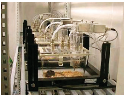
Apparatus for measuring whole-body metabolism in small animals.
