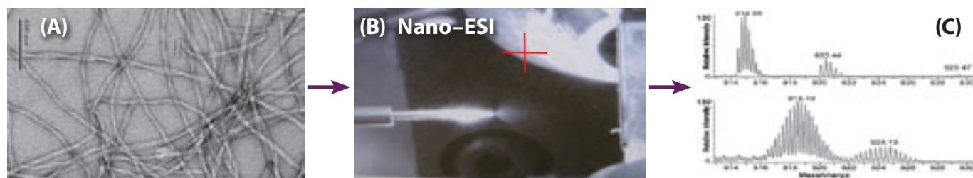
(A) Electron micrograph image of amyloid fibrils. Amyloid fibrils are electrosprayed (B) into the mass spectrometer and number of backbone amide protons exchanging with deuterium are measured in an ESI spectrum (C).
